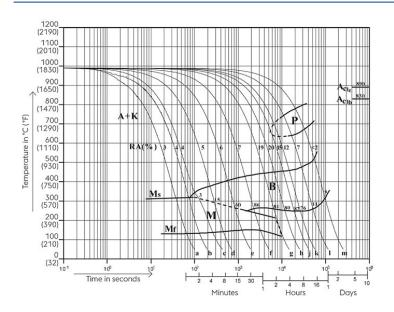
Austenitising temperature: 1025°C (1877°F) Holding time: 15 minutes 5...100 phase percentages 0.5...180 cooling parameter, i.e. duration of cooling from 800 - 500°C (1472-932°F) in s  $\times$  10<sup>-2</sup>
