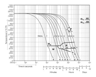
Austenitising temperature:  $1020^{\circ}\text{C}$  ( $1868^{\circ}\text{F}$ ) Holding time: 15 minutes 5...100 phase percentages 0.5...180 cooling parameter, i.e. duration of cooling from 800 -  $500^{\circ}\text{C}$  (1472- $932^{\circ}\text{F}$ ) in s x  $10^{-2}$
