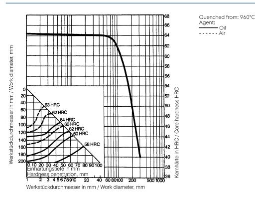
Influence of work diameter on core hardness and hardness penetration
