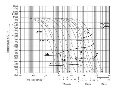
Austenitising temperature: 990°C (1814°F) Holding time: 15 minutes 5...100 phase percentages 0.15...400 cooling parameter, i.e. duration of cooling from 800 - 500°C (1472-932°F) in s x  $10^{-2}$
