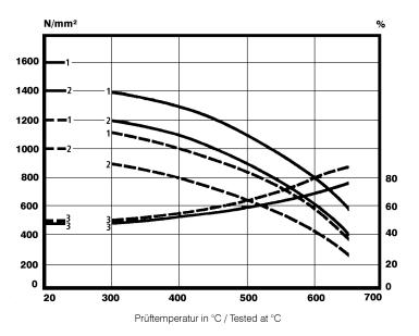
heat treated 1600 N/mm<sup>2</sup> heat treated 1200 N/mm<sup>2</sup> heat treated 1200 N/mm<sup>2</sup> ... Tensile strength N/mm<sup>2</sup> ... 0.2% proof stress N/mm<sup>2</sup> 3... Reduction of area %
