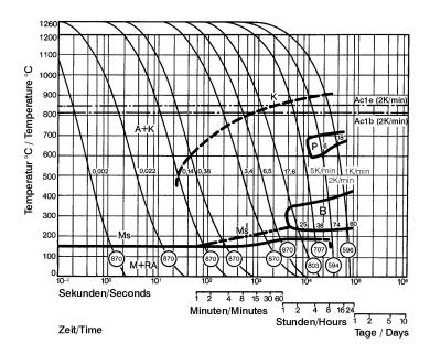
Austenitising temperature:  $1260^{\circ}\text{C}$  ( $2300^{\circ}\text{F}$ ) Holding time: 150 seconds
