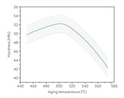
Heat Treatment for optimum properties: Solution Annealing: 1000°C / 1h soaking time / air cooling to room temperature Ageing: 500°C / 3h soaking time / air cooling
