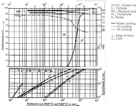
HV10... Vickers Hardness K... Carbide RA... Residual austenite M... Martensite P... Perlite
