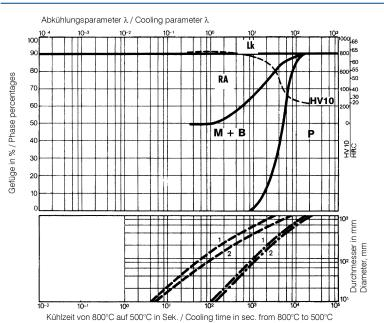
HV10... Vickers Hardness Lk... Ledeburite carbide RA... Residual austenite M... Martensite B... Bainite P... Perlite
